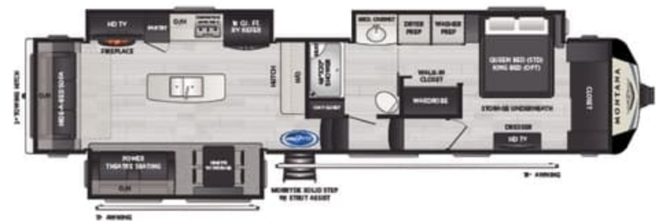
3812/3813MS | Rear living room w/ master suite & walk-in closet W/ REFRIGERATOR RES. REFRIGERATOR WEIGHT:13635 LENGTH:40' 9"
