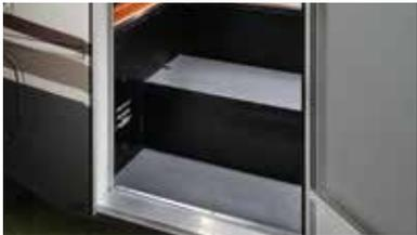
Sunseeker's entry step is integrated into the sidewall. No more slippery, or damaged power steps. (N/A MBS)
