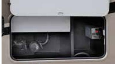
Heated/enclosed holding tanks use warm air from the furnace to protect tanks and valves. (N/A 2250SLE, 2550DSLE, MBS and Transit)
